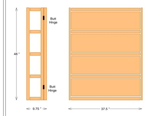
All wood is 3/4 " clear or select pine. Biskit joined at ends. Shelves are held with dowels. A short peg is attached to side rails for shelf support. Two pairs of butt hinges allow sides to be folded after shelves are folder in upright position.
